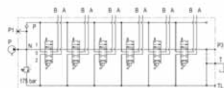
Schematic of standard 6-spool (VDM6/DDDDDD/U4S)
