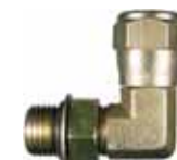
Brennan 6809-NWO Male SAE O-Ring Boss / Female 37° Flare Swivel 90° Elbow Page 1160
