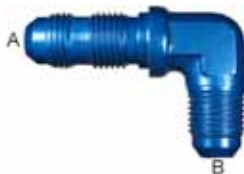
Male 37° Flare / Male 37° Flare 90° Bulkhead Union Elbow Blue Anodized Alum (AN 833)
