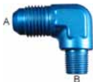
Male 37° Flare / Male Pipe 90° Elbow Aluminum (AN 822)
