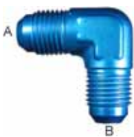
Male 37° Flare / Male 37° Flare 90° Elbow, Blue Anodized Aluminum (AN 821)
